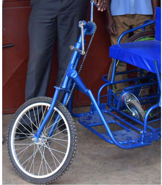
(Figure 4.2) This image displays the newer prototype that local Uganda manufacturers created. It has a smaller wheel dimension of 20".
