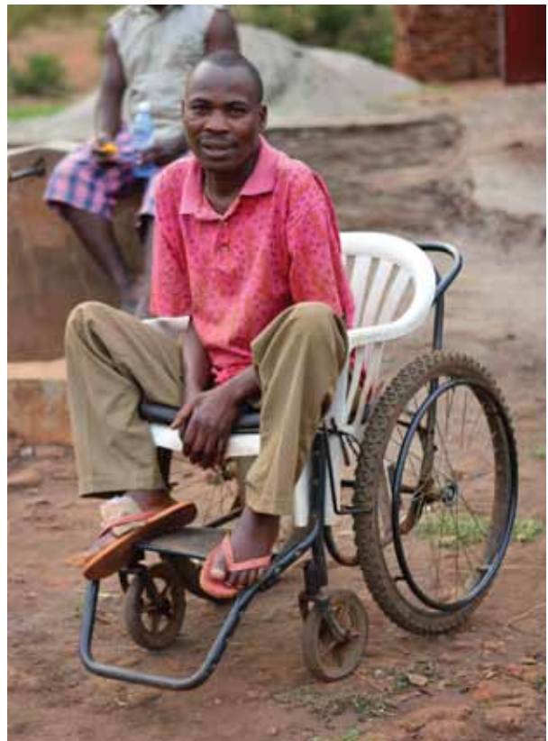
A man who had a simple, but not a long term solution to repairing a imported wheelchair when his chair broke.
